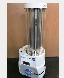
Disinfecting robot mounted with an ultraviolet light irradiator
