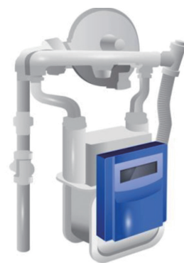
Gas meter installed with a seismic sensor
